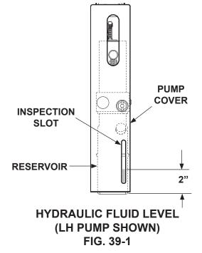
2. If needed, add fluid to the reservoir as follows. Unbolt the pump cover as shown in FIG. 39-2.
